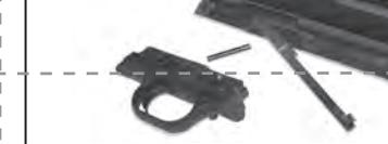
**3** With safety on, install trigger group by first inserting front up into the receiver and then swinging rear of group up and into the receiver. **DO NOT** pull trigger during install.
