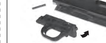
**4** Reinstall drift pin(s) through receiver to secure trigger group.
